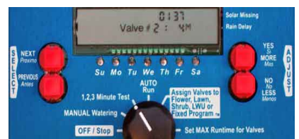
Figure 5: 1,2,3 Minute Test selected by rotary switch. YES/MORE switch was pushed to select 004Minute test. Valve #2 has run 1 min + 37 sec. Solar sensor is missing or connected backwards. Rain sensor is missing or has detected rain.
