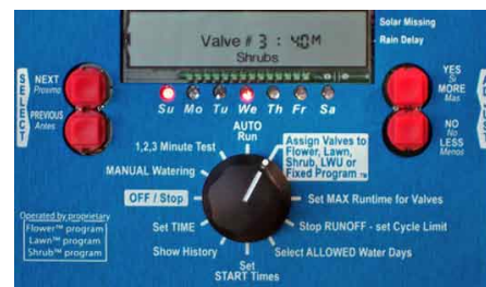
Figure 9: Set MAX Runtime is selected by rotary switch. Display shows that MAX Runtime is set to 40 Minutes for Valve#3. Any Runtime from 0 to 255 may be set.
