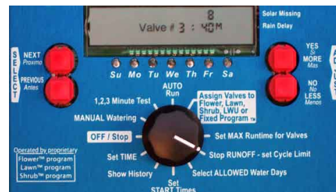
Figure 10: Stop RUNOFF is selected by rotary switch. Display shows that MAX Runtime of 40 minutes is limited to 8 minutes cycles each hour. So, five hours will be required to deliver 40 minutes of water each watering day.
