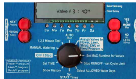
Figure 10: Stop RUNOFF is selected by rotary switch. Display shows that MAX Runtime of 40 minutes is limited to 8 minutes cycles each hour. So, five hours will be required to deliver 40 minutes of water each watering day.
