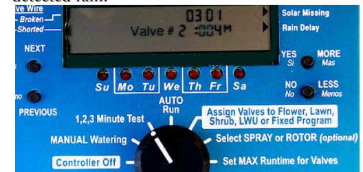
Figure 15: 1,2,3 Minute Test selected by rotary switch. MORE switch was pushed to select 004Minute test. Valve #2 has run 03 min + 01 sec. Solar sensor is missing or connected backwards. Rain sensor is missing or has detected rain.
