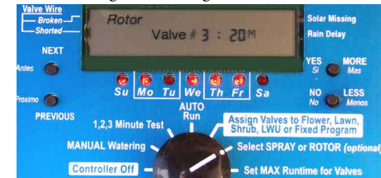
Figure 8: Optional Select SPRAY or ROTOR selected by rotary switch. Display shows that Rotor is assigned to Valve 3. Also shown 20 minute Runtime that goes with assignment of Rotor.
