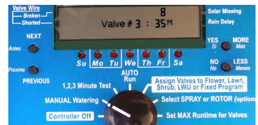
Figure 15: 1,2,3 Minute Test selected by rotary switch. MORE switch was pushed to select 004Minute test. Valve #2 has run 03 min + 01 sec. Solar sensor is missing or connected backwards. Rain sensor is missing or has detected rain.
