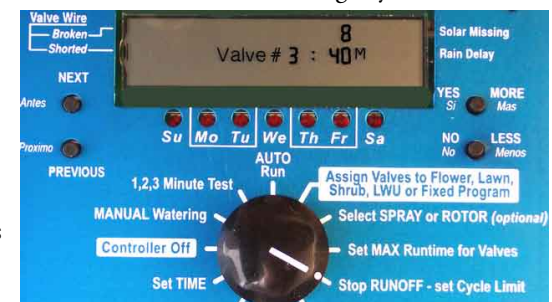
Figure 10: Stop RUNOFF is selected by rotary switch. Display shows that MAX Runtime of 40 minutes is limited to 8 minutes cycles each hour. So, five hours will be required to deliver 40 minutes of water each watering day.
