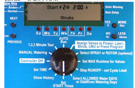
Figure 14: Manual Watering is selected by rotary switch. NEXT switch was pushed to select Valve#3. YES switch was pushed to select it. Valve #3 has MAX Runtime of 40 minutes (see Figure 9). But SFR has signalled need for only 35 minutes of water. Cycle limit is 8minute/hour.
