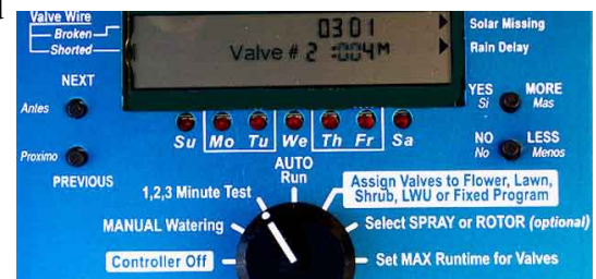
Figure 5: 1,2,3 Minute Test selected by rotary switch. YES/MORE switch was pushed to select 004Minute test. Valve #2 has run 03 min + 01 sec. Solar sensor is missing or connected backwards. Rain sensor is missing or has detected rain.
