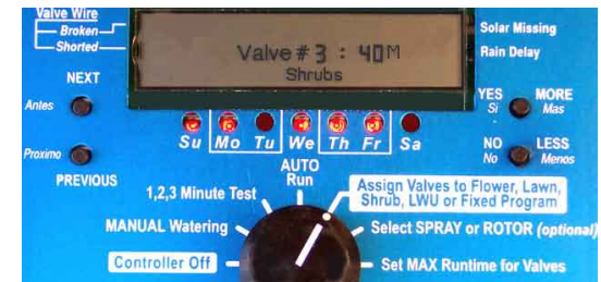
Figure 7: Assign Valves to Flower™, Lawn™, Shrub™, LWU or Fixed programs selected by rotary switch. Display shows that Valve 3 is assigned to Shrub™ program. Also shown are the Water Days for the program under current weather.
