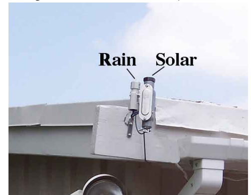
Figure 2: SFR sensor mounted along roof. This mounting of the sensor gives accurate solar readings from sunrise to end of day.
